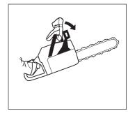
3 You can also use the chain brake as a temporary brake when you change position or if you put the saw down for a short time. You should also apply the chain brake manually if there is a risk of the chain accidentally hitting anyone or anything close by.
